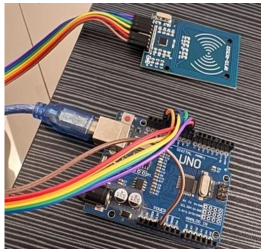
Figure 6. Integration of Arduino and RFID Module
